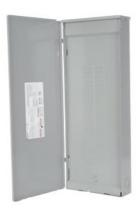
SIEMENS LOW VOLTAGE ES SERIES LOAD CENTER. MAIN LUG WITH 42 1-Inch Spaces ALLOWING MAX 60 CIRCUITS. 1-PHASE 3-WIRE SYSTEM RATED 120/240V(225A) 100KA INTERRUPT. SPECIAL FEATURES: ALUMINUM BUS, GRAY TRIM, NEMA TYPE3R ENCLOSURE FOR OUTDOOR USE. REPLACED BY SNW4264L1225. AVAILABLE 4/1/2020
