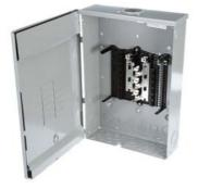
SIEMENS LOW VOLTAGE ES SERIES LOAD CENTER. MAIN LUG WITH 12 1-Inch Spaces ALLOWING MAX 24 CIRCUITS. 1-PHASE 3-WIRE SYSTEM RATED 120/240V(125A) 100KA INTERRUPT. SPECIAL FEATURES: ALUMINUM BUS, GRAY TRIM, NEMA TYPE3R ENCLOSURE FOR OUTDOOR USE. REPLACED BY SNW1224L1125. AVAILABLE 4/1/2020
