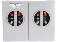
Siemens Low Voltage Talon Meter Sockets Residential - Talon Meter Sockets UAS8/9 Aluminum are Residential Enclosures Single-Family Metering. Type: UAS8/9 Features: NO BYPASS Application: RESIDENTIAL Std: UL V. Rating: 300V A. Rating: 100A Phase: 1 OR 3 PHASE Size: 5.5 x 16.6 x 21.0 No Of Cutouts: 10 Cutout Size: 2 x 2.750, 6 x (1, 1-1/4, 1-1/2, 2), 2 x (1/2, 3/4, 1, 1-1/4, 1-1/2) Cable Entry: OH Terminals: 5. Surface mounting. Operating Temperature: Avg AMBIENT Enclosure: AL
