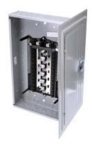
SIEMENS LOW VOLTAGE ES SERIES LOAD CENTER. MAIN LUG WITH 24 1-Inch Spaces ALLOWING MAX 40 CIRCUITS. 1-PHASE 3-WIRE SYSTEM RATED 120/240V(125A) 100KA INTERRUPT. SPECIAL FEATURES: ALUMINUM BUS, GRAY TRIM, NEMA TYPE1 ENCLOSURE FOR INDOOR USE. REPLACED BY SN2448L1125. AVAILABLE 4/1/2020
