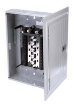
SIEMENS LOW VOLTAGE ES SERIES LOAD CENTER. MAIN LUG WITH 20 1-Inch Spaces ALLOWING MAX 24 CIRCUITS. 1-PHASE 3-WIRE SYSTEM RATED 120/240V(125A) 100KA INTERRUPT. SPECIAL FEATURES: ALUMINUM BUS, FACTORY INSTALLED GROUND BAR, GRAY TRIM, NEMA TYPE1 ENCLOSURE FOR INDOOR USE. REPLACED BY SN2040L1125. AVAILABLE 4/1/2020
