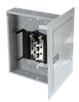
SIEMENS LOW VOLTAGE ES SERIES LOAD CENTER. MAIN LUG WITH 12 1-Inch Spaces ALLOWING MAX 24 CIRCUITS. 1-PHASE 3-WIRE SYSTEM RATED 120/240V(125A) 100KA INTERRUPT. SPECIAL FEATURES: ALUMINUM BUS, GRAY TRIM, NEMA TYPE1 ENCLOSURE FOR INDOOR USE. REPLACED BY SN1224L1125. AVAILABLE 4/1/2020
