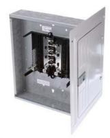
SIEMENS LOW VOLTAGE ES SERIES LOAD CENTER. MAIN LUG WITH 12 1-Inch Spaces ALLOWING MAX 12 CIRCUITS. 1-PHASE 3-WIRE SYSTEM RATED 120/240V(125A) 100KA INTERRUPT. SPECIAL FEATURES: ALUMINUM BUS, GRAY TRIM, NEMA TYPE1 ENCLOSURE FOR INDOOR USE. REPLACED BY SN1212L1125. AVAILABLE 4/1/2020
