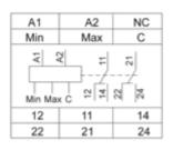
A1,A2 : Supply voltage Max : High level Min : Low level C : References or Tank earth electrode 11-14,12 : 1st C/O contact of output relay 21-24,22 : 2nd C/O contact of output relay
