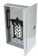
SIEMENS LOW VOLTAGE RISER LOAD CENTER. MAIN LUG WITH 16 1-INCH SPACES ALLOWING MAX 32 CIRCUITS. 1-PHASE 3-WIRE SYSTEM RATED 120/240V (125A) 100KA INTERRUPT. SPECIAL FEATURES: ALUMINUM BUS, INTERCHANGEABLE MAIN, GRAY TRIM.
