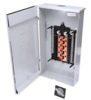
SIEMENS LOW VOLTAGE PL SERIES LOAD CENTER. MAIN LUG WITH 20 1-Inch Spaces ALLOWING MAX 30 CIRCUITS. 1-PHASE 3-WIRE SYSTEM RATED 120/240V(150A) 100KA INTERRUPT. SPECIAL FEATURES: COPPER BUS, INTERCHANGEABLE MAIN, GRAY TRIM, NEMA TYPE3R ENCLOSURE FOR OUTDOOR USE. REPLACED BY PNW2040L1150C. AVAILABLE 4/1/2020
