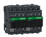
Reversing Contactor, TeSys Deca, 3P(3NO), AC-3, <=440V, 9A, 110V AC 50/60Hz coil, screw clamp terminals
