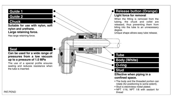
Optimum piping in less space with 20% reduction of the outside
