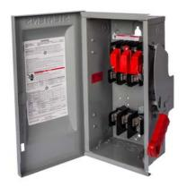
Siemens Low Voltage Circuit Protection Heavy Duty Safety Switches - Type ENCLOSED / SAFETY SWITCH Meets stds: UL. Built material: 316SSsingle throw action. Rated 600V (100 A) at 60Hz.3-Pole. Insulated. TYPE 4X enclosure with 2 or 3 point mounting. No special features listed.
