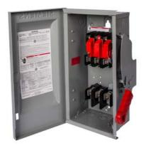
Siemens Low Voltage Circuit Protection Heavy Duty Safety Switches. Type: ENCLOSED, SAFETY SWITCH Std: UL V. Rating: 240V A. Rating: 30 A No. Of Poles: 3P F. Rating: 60Hz Action: SINGLE THROW Material: SS Enclosure: TYPE 4X. 2-3 point mounting holes. Insulation: YES O. Cycles: 10000 O. Temperature: (-20F-120F) AMBIENT TEMPERATURE Environmental Conditions: INDUSTRIAL CORROSIVE RESISTANCE
