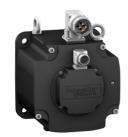
servo motor BMH, Lexium 32, 30Nm, 5000rpm, keyed shaft, with brake, IP65, IP67, 128 multiturn encoder
