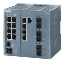
SCALANCE XB213-3 managed Layer 2 IE switch 13x 10/100 Mbit/s RJ45 ports, 3x MM FO ST port 1x console port, diagnostics LED, redundant power supply, IEC 62443-4-2 certified; temperature range 0 °C to +60 °C; DIN-rail mounting; default EtherNet/IP.
