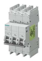
Miniature circuit breaker 240 V 10kA, 3-pole, D, 32 A, D=70 mm according to UL 489  $\,$
