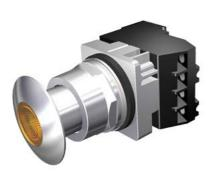
30mm Command/52, Chrome Finish Heavy Duty,Watertight/Oiltight Complete Metal Unit Illuminated Push-Pull Operator Transformer type, 120V AC LED Lamp Mushroom Head Cap Small 1 3/4" (44.5 mm) Metal, Chrome with Amber Lens 2 Position Maintained, Pull-to-Release with 1 N.O. - 1 N.C. Heavy Duty Contacts, A600/P600 UL Listed, CSA Certified NEMA 1,3,3R,4,4X,12,13 & Automotive Standards
