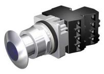
30mm Command/52, Chrome Finish Heavy Duty, Watertight/Oiltight Complete Metal Unit Illuminated Push-Pull Operator Transformer type, 120V AC Incandescent Lamp Mushroom Head Cap Small 1 3/4" (44.5 mm) Metal, Chrome with Blue Lens 2 Position Maintained, Pull-to-Release with 2 N.O. - 2 N.C. Heavy Duty Contacts, A600/P600 UL Listed, CSA Certified NEMA 1,3,3R,4,4X,12,13 & Automotive Standards
