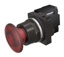
30mm BlackMax, Epoxy Coated Corrosion Resistant Complete Metal Unit Illuminated Push-Pull Operator Transformer type, 600V AC LED Lamp Mushroom Head Cap Small 1 3/4" (44.5 mm) Plastic, Red 3 Position Momentary UL Listed, CSA Certified NEMA 1,3,3R,4,4X,12,13 & Automotive Standards
