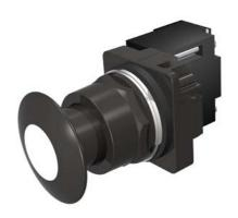
30mm BlackMax, Epoxy Coated Corrosion Resistant Complete Metal Unit Illuminated Push-Pull Operator Transformer type, 600V AC Incandescent Lamp Mushroom Head Cap Small 1 3/4" (44.5 mm) Metal, Black with White Lens 3 Position Momentary UL Listed, CSA Certified NEMA 1,3,3R,4,4X,12,13 & Automotive Standards
