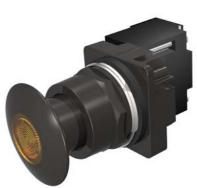
30mm BlackMax, Epoxy Coated Corrosion Resistant Complete Metal Unit Illuminated Push-Pull Operator Transformer type, 600V AC LED Lamp Mushroom Head Cap Small 1 3/4" (44.5 mm) Metal, Black with Amber Lens 3 Position Momentary UL Listed, CSA Certified NEMA 1,3,3R,4,4X,12,13 & Automotive Standards
