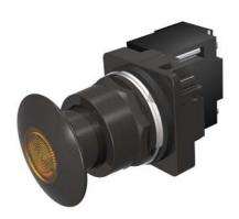
30mm BlackMax, Epoxy Coated Corrosion Resistant Complete Metal Unit Illuminated Push-Pull Operator Transformer type, 600V AC Incandescent Lamp Mushroom Head Cap Small 1 3/4" (44.5 mm) Metal, Black with Amber Lens 3 Position Momentary UL Listed, CSA Certified NEMA 1,3,3R,4,4X,12,13 & Automotive Standards
