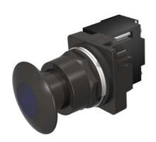
30mm BlackMax, Epoxy Coated Corrosion Resistant Complete Metal Unit Illuminated Push-Pull Operator Transformer type, 600V AC Incandescent Lamp Mushroom Head Cap Small 1 3/4" (44.5 mm) Metal, Black with Blue Lens 3 Position Momentary UL Listed, CSA Certified NEMA 1,3,3R,4,4X,12,13 & Automotive Standards
