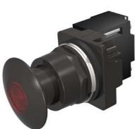
30mm BlackMax, Epoxy Coated Corrosion Resistant Complete Metal Unit Illuminated Push-Pull Operator Transformer type, 600V AC Incandescent Lamp Mushroom Head Cap Small 1 3/4" (44.5 mm) Metal, Black with Red Lens 3 Position Momentary UL Listed, CSA Certified NEMA 1,3,3R,4,4X,12,13 & Automotive Standards
