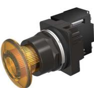
30mm BlackMax, Epoxy Coated Corrosion Resistant Complete Metal Unit Illuminated Push-Pull Operator Transformer type, 480V AC Incandescent Lamp Mushroom Head Cap Small 1 3/4" (44.5 mm) Plastic, Amber 3 Position Momentary UL Listed, CSA Certified NEMA 1,3,3R,4,4X,12,13 & Automotive Standards
