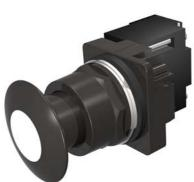
30mm BlackMax, Epoxy Coated Corrosion Resistant Complete Metal Unit Illuminated Push-Pull Operator Transformer type, 480V AC LED Lamp Mushroom Head Cap Small 1 3/4" (44.5 mm) Metal, Black with White Lens 3 Position Momentary UL Listed, CSA Certified NEMA 1,3,3R,4,4X,12,13 & Automotive Standards
