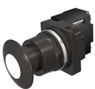
30mm BlackMax, Epoxy Coated Corrosion Resistant Complete Metal Unit Illuminated Push-Pull Operator Transformer type, 480V AC Incandescent Lamp Mushroom Head Cap Small 1 3/4" (44.5 mm) Metal, Black with White Lens 3 Position Momentary UL Listed, CSA Certified NEMA 1,3,3R,4,4X,12,13 & Automotive Standards
