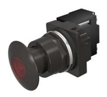
30mm BlackMax, Epoxy Coated Corrosion Resistant Complete Metal Unit Illuminated Push-Pull Operator Transformer type, 480V AC LED Lamp Mushroom Head Cap Small 1 3/4" (44.5 mm) Metal, Black with Red Lens 3 Position Momentary UL Listed, CSA Certified NEMA 1,3,3R,4,4X,12,13 & Automotive Standards
