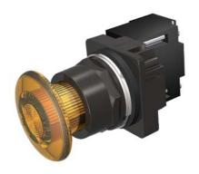
30mm BlackMax, Epoxy Coated Corrosion Resistant Complete Metal Unit Illuminated Push-Pull Operator Transformer type, 240V AC Incandescent Lamp Mushroom Head Cap Small 1 3/4" (44.5 mm) Plastic, Amber 3 Position Momentary UL Listed, CSA Certified NEMA 1,3,3R,4,4X,12,13 & Automotive Standards
