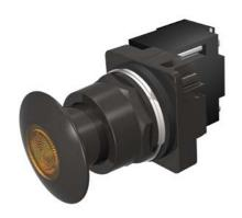
30mm BlackMax, Epoxy Coated Corrosion Resistant Complete Metal Unit Illuminated Push-Pull Operator Transformer type, 240V AC LED Lamp Mushroom Head Cap Small 1 3/4" (44.5 mm) Metal, Black with Amber Lens 3 Position Momentary UL Listed, CSA Certified NEMA 1,3,3R,4,4X,12,13 & Automotive Standards
