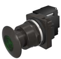
30mm BlackMax, Epoxy Coated Corrosion Resistant Complete Metal Unit Illuminated Push-Pull Operator Transformer type, 240V AC LED Lamp Mushroom Head Cap Small 1 3/4" (44.5 mm) Metal, Black with Green Lens 3 Position Momentary UL Listed, CSA Certified NEMA 1,3,3R,4,4X,12,13 & Automotive Standards
