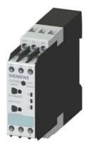
Insulation monitoring relay for ungrounded (IT) supply systems up to 250 V AC, 15-400 Hz and up to 300 V DC Measuring range 1-100 kohm Supply voltage 24-240 V AC/DC 22.5 mm, 1 change-over contact screw terminal
