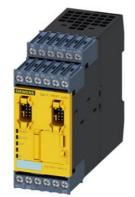
Fail-safe digital module DM-F PROFIsafe, for fail-safe shutdown via bus/PROFIsafe, Us: 24 V DC, 2 relay enabling circuits, 2 relay outputs, 3 inputs, maximum achievable SIL IEC 61508: 3, maximum achievable PL ISO 13849-1: E
