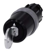
key-operated switch Siemens, 22 mm, round, plastic with metal front ring, lock number SSG10, with 2 keys, 3 switch positions I>O<II, momentary contact on the left, latching on the right, actuating angle 2x45°, 10:30h/12h/13:30h, key removal O
