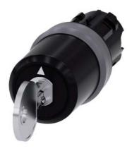
key-operated switch Siemens, 22 mm, round, plastic with metal front ring, lock number SSG10, with 2 keys, 3 switch positions I-O-II, latching, actuating angle 2x45°, 10:30h/12h/13:30h, key removal II
