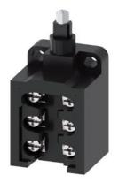
Position switch Plastic enclosure open type 30 mm 2 NO/1 NC slow-action contacts Metal plunger, IP10  $\,$
