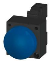
22MM PLASTIC ROUND COMPLETE UNIT COMBINATION: INDICATOR LIGHT WITH CONCENTRIC RINGS ILLUMINATED WITH INTEGRATED LED 24V AC/DC SCREW TERMINAL WITH HOLDER BLUE !!! Phased-out product !!! SIRIUS ACT 3SU1 is successor Preferred successor type is >>3SU1102-6AA50-1AA0<<
