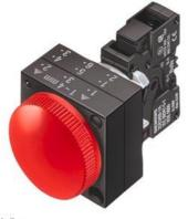
22MM PLASTIC ROUND COMPLETE UNIT COMBINATION: INDICATOR LIGHT WITH SMOOTH LENSE ILLUMINATED WITH INTEGRATED LED 24V AC/DC SPRING-LOADED TERMINAL WITH HOLDER RED !!! Phased-out product !!! SIRIUS ACT 3SU1 is successor Preferred successor type is >> 3SU1102-6AA20-3AA0<
