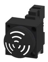
Acoustic signal device, 22 mm, round, plastic, black, continuous tone 2.4 kHz, IP65, sound pressure min. 80 dB/10 cm, with holder, lampholder BA 9S, operating voltage 24 V AC/DC, screw terminal !!! Phased-out product !!! Successor is SIRIUS ACT 3SU1 Preferred successor type is >>3SU1200-6KB10-1AA0<<
