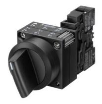
Toggle switch, 22 mm, round, plastic, black, knob, short, 2 switch positions O-I, latching, actuating angle 50 degrees, 11/1 o'clock, with holder, 1 NO, screw terminal !!! Phased-out product !!! Successor is SIRIUS ACT 3SU1 Preferred successor type is >>3SU1002-2BF10-0AA0 + 3SU1400-1AA10-1BA0 + 3SU1500-0AA10-0AA0<<
