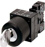
RONIS KEY-OPERATED SWITCH 22MM, ROUND, PLASTIC, LOCK NUMBER SB 30, WITH 2 KEYS, 2 SWITCH POSITIONS O-I LATCHING, ACTUATING ANGLE 50 DEGREES, 1200/1400 HOURS, REMOVE KEY O+I, WITH HOLDER, 1NO+1NC, SCREW CONNECTION, POSSIBLE SPECIAL LOCKS: SB31, 421, 455 !!! Phased-out product !!! SIRIUS ACT 3SU1 is successor Preferred successor type is >>3SU1100-4BF11-1FA0<<
