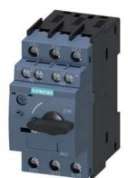
Circuit breaker size S00 for transformer protection A-release 2.8...4 A N-release 82 A screw terminal Standard switching capacity with transverse auxiliary switches 1 NO+1 NC  $\,$
