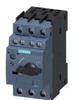
Circuit breaker size S00 for transformer protection A-release 1.4...2 A N release 42 A screw terminal Standard switching capacity with transverse auxiliary switches 1 NO+1 NC  $\,$
