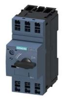
Circuit breaker size S00 for transformer protection A-release 0.45...0.63 A N-release 13 A Spring-type terminal Standard switching capacity
