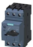
Circuit breaker size S00 for transformer protection A-release 0.45...0.63 A N-release 13 A screw terminal Standard switching capacity
