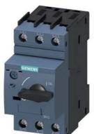
Circuit breaker size S00 for transformer protection A-release 0.18...0.25 A N-release 5.2 A screw terminal Standard switching capacity
