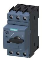
Circuit breaker size S00 for transformer protection A-release 0.14...0.2 A N-release 4.2 A screw terminal Standard switching capacity
