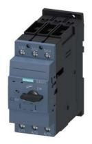
Circuit breaker size S2 for starter combination Rated current 40 A N-release 585 A screw terminal Standard switching capacity
