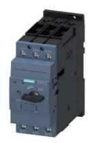
Circuit breaker size S2 for starter combination Rated current 25 A Nrelease 325 A Screw terminal Standard switching capacity
